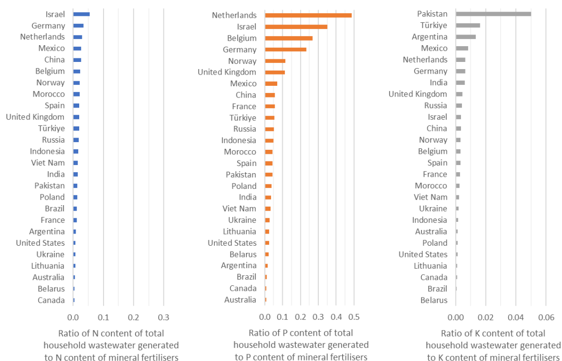
Figure 5.3. Potential of household wastewater to replace mineral fertilisers used in agricultural production for N, P and K in selected major 26 countries, 2021
