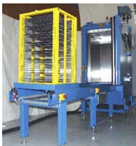
Figure 5.7: Example of release measurement facility: Front part: conveyor with material to be measured (box), background: measurement chamber with detectors (floor, ceiling, both side walls and doors) surrounding the material
