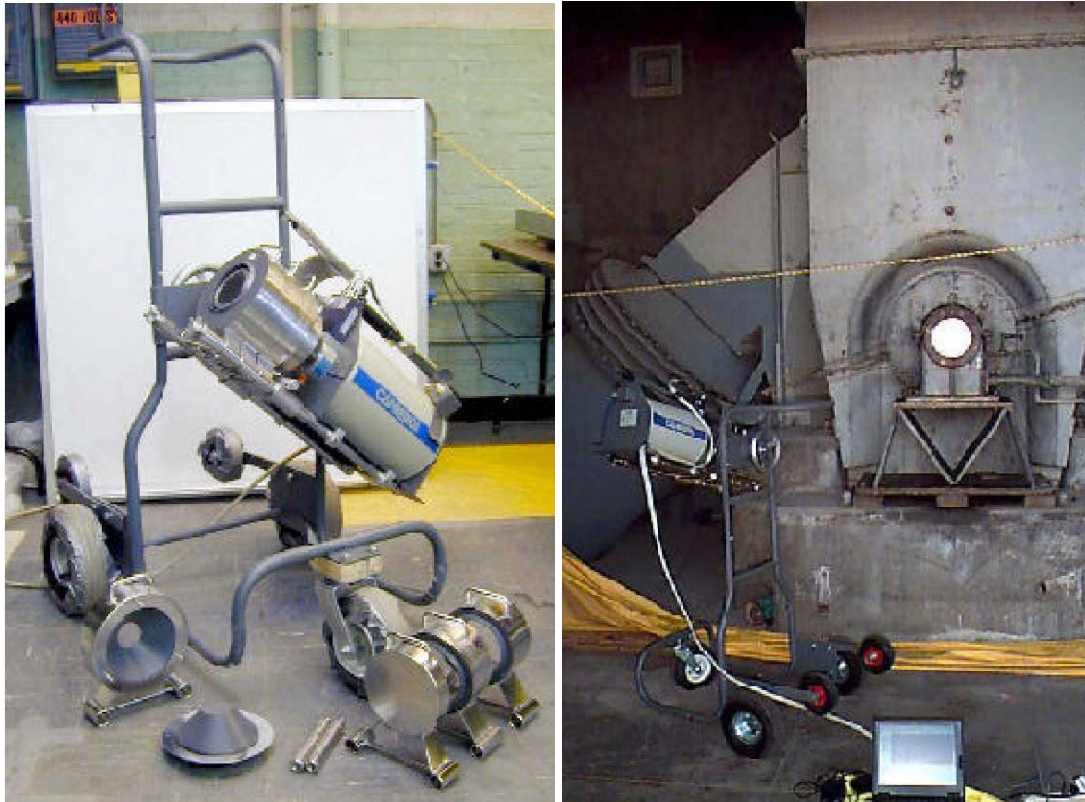
Figure 5.2: The ISOCS system in preparation for use (left) and in use at the fan building of the Brookhaven Graphite Research Reactor
