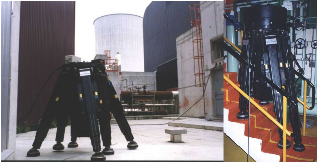
Figure B.6. Sherpa transporter robot, in Chooz-B (1993, left) and Trino (1994, right)
