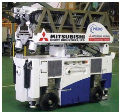
Figure E.1.24. Remote heavy load unloading cart for narrow areas (Super Giraffe)
