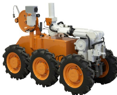
Figure B.27. Emergency response robot
