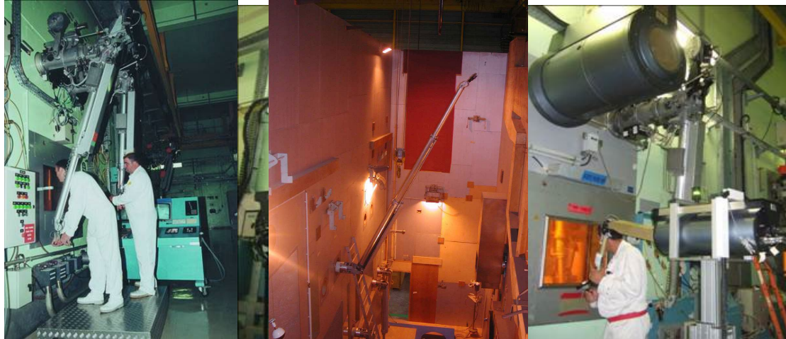
Figure B.42. A typical workstation at the Orano La Hague reprocessing plant (left); the MT200 TAO telerobot in a ceiling work configuration in an Orano test cell (centre); a mixed workstation in a controlled area showing the MT200 TAO telerobot operated by the master arm MAT6D (Haption™) and a standard mechanical telemanipulator MT200 (right).
