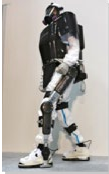
Figure E.1.27. Worker wearing a work-assist robot for disaster response
