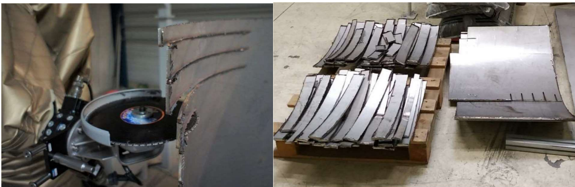
Figure B.40. Cutting of shuttle drums and endurance test of the robot - tool - consumable combination.
