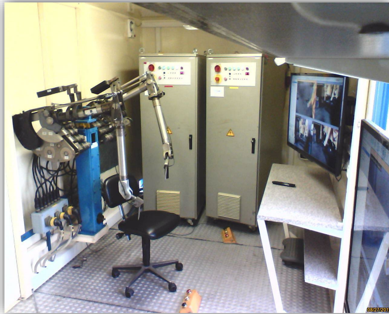
Figure B.29. Master arms installed in 20' ISO container (see next figure)
