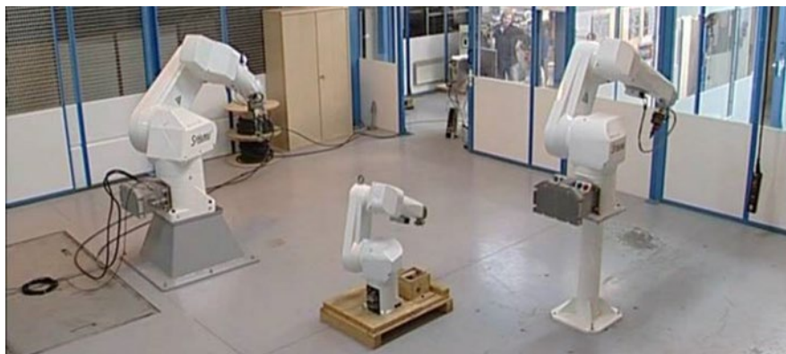
Figure B.32. Stäubli™ RX90, 130 and 170 range of radiation tolerant industrial robots implemented by AREVA NC (Orano La Hague)
