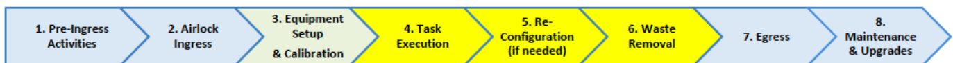
Figure E.2.2. Simplified process flowchart for robotic and automation operations inside the vault.
