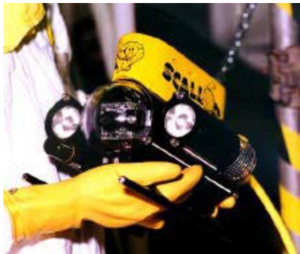
Figure B.2. Scallop Remotely Operated Underwater Vehicle (EPRI, 2015)
