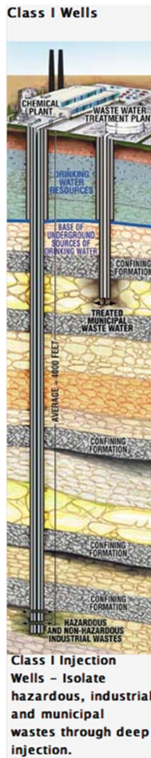
Figure 5.4-3: Deep well injection techniques for hazardous and toxic waste fluids ( http://water.epa.gov/type/groundwater/uic/wells_class1.cfm#what_is )
