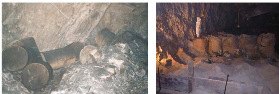
Figure 5.1-1: Some pictures of the waste inventory inside the galleries of the chalk mine of St-Ursanne, archive of the DMS-project of the Canton of Jura (on the left are some of the thousands empty or filled drums dumped into the mine between 1970 and 1993, and on the right: big-bags with galvanic waste emplaced in 1995)
