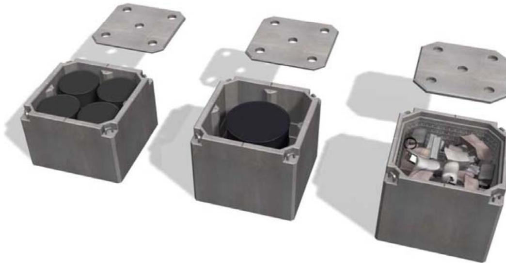
Figure 3.5: Schematic view of the Type I (left), Type II (centre) and Type III (right) caissons containing different waste types (ONDRAF/NIRAS 2011f)
