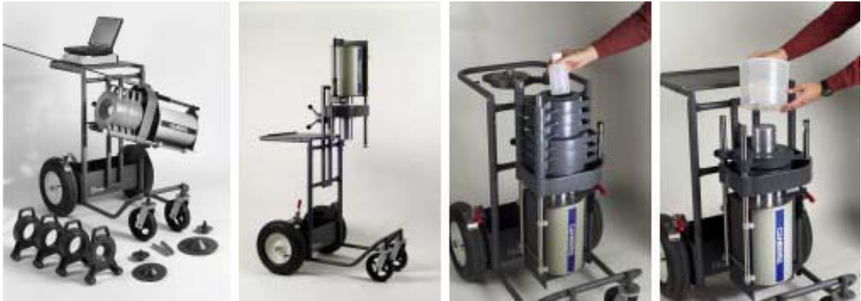
Figure: 4.3 Isocs In-situ Gamma Spectrometer
