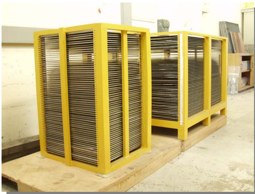
Figure 2: Calibration racks for release measurements facilities
