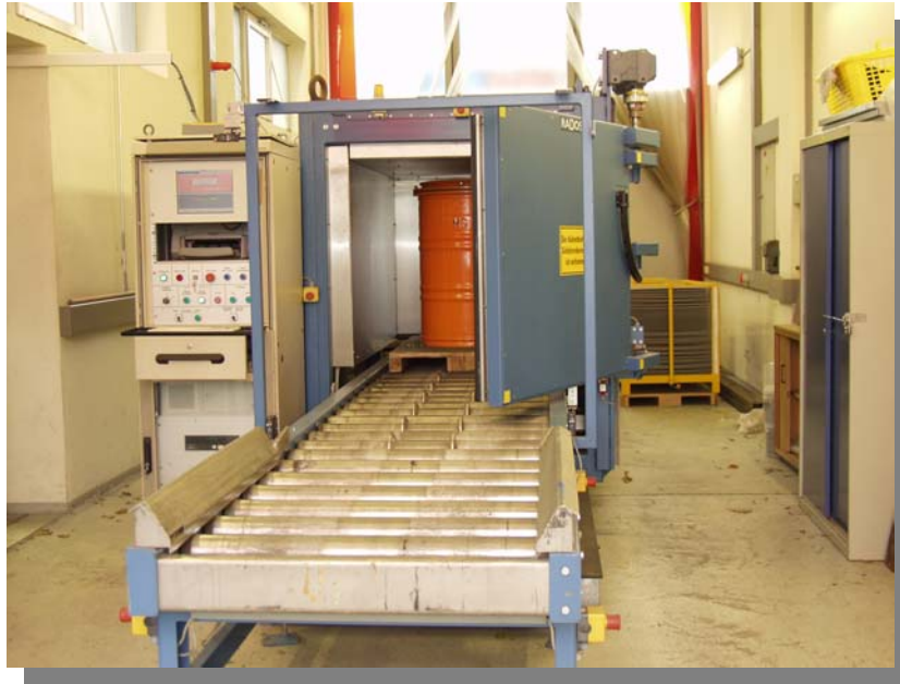
Figure 1: Release measurement facility
