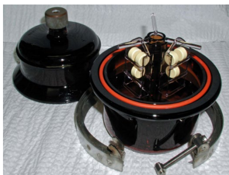
Figure 3.8. Irradiation vessel (shown post-irradiation and with coupons and holders)
