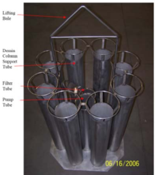
Figure 31: Tri Nuclear Submersable Demineraliser Configuration
