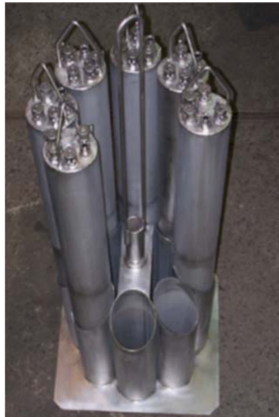
Figure 31: Tri Nuclear Submersable Demineraliser Configuration
