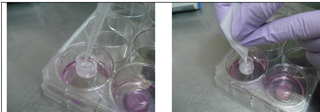
[Figure 4] Application of solids; First, apply 40 \mu\text{L} of DPBS for wetting the surface of the insert (left), and then apply the weighed test chemical to the insert.
