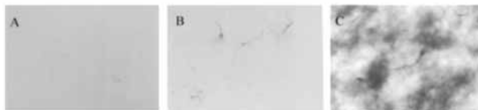
Fig. 1. Microscopic views of SWCNT suspensions ( \times 400 ). (A) 0.125 mg/kg bw/day (0.00625 mg/ml); (B) 1.25 mg/kg bw/day (0.0625 mg/ml); (C) 12.5 mg/kg bw/day (0.625 mg/ml).
