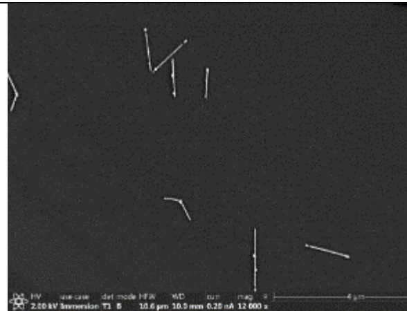
Figure 152: SEM 7, electron beam voltage 2 kV, Detector: BSE, Pixel size: 3.54 nm/ px.
