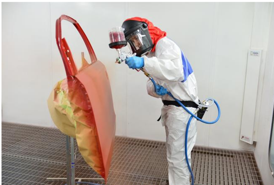
Figure 5.2. Applying Paint in the Automotive Industry
