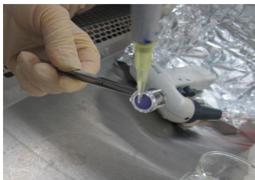
[Figure 7] Removal of MTT from inside/outside of the insert after MTT treatment
