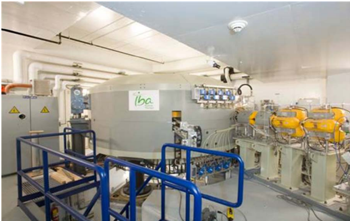
Figure 5. A commercial medical cyclotron, the Proteus 235 by Ion Beam Applications S.A. (IBA). It produces a proton beam with a fixed energy of 250 MeV. The diameter of the accelerator is 2.5 metres, one tenth the size of the CNAO synchrotron ring
