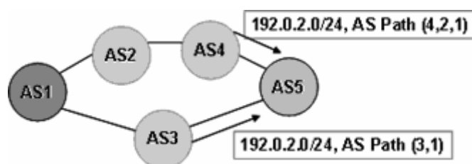
Figure 6: Inter-domain routing with Autonomous System Numbers and Prefixes
